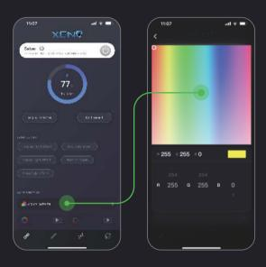
Pictured here is the Color Palette. This allows the user to select the color manually, from pressing on the color, or by entering an RGB value from 0-255 fir each color (Red, Green, and Blue).
