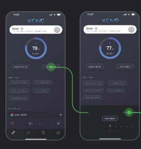
• Press Font Select from the main screen to select a font from those currently installed on the saber. After selecting a font, you'll have the option to edit the light effect of the saber for that selected font by pressing 'Setting light effect'. Hum light effect changes the basic lightstyle, from options like fire blade, unstable and pulse; Saber Mode selects the use of the blade, such as Ghost Blade or Blaster mode. Reset light effect returns the fonts light effects to a default setting.
